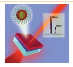
By exploiting sol-gel chemistry and the nanoimprinting process, a low-cost up-converted distributed feedback laser is realized. Properly synthesized graded CdSe-CdZnS-ZnS quantum dots are used as active gain material. The laser prototype efficiently works in the visible region, by pumping with one- or two-photon processes. This solution-processed device opens the way to the production of emission-tunable compact lasers.
