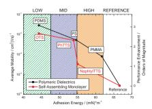
Dielectric surface modifications can improve the performance of organic thinfilm transistors (OTFTs) significantly. Devices utilizing tailored dielectric surface modifications based on polymers and trichlorosilane-terminated self-assembled monolayers have been produced. The application of these novel dielectric surface modifications facilitates perylene thin-films with a superior film quality and high-performance perylene based OTFTs with a high charge-carrier mobility.
